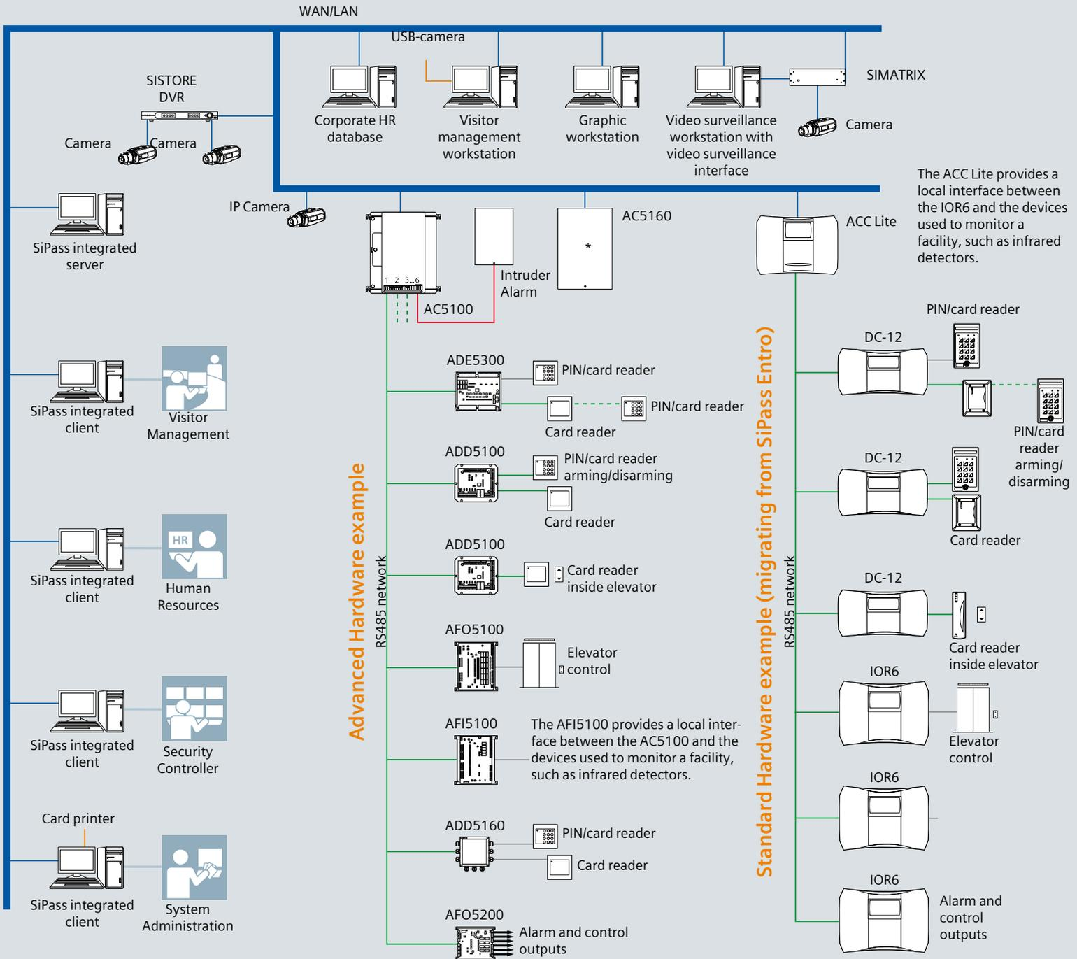
\* One of the six ports on the AC5100 is a multi-purpose IS interface that can be used for Intruder, high-level elevator control, Securitel or, if none of these are in use, for any other FLN.
